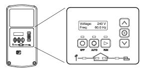
The RDC2 controller provides integrated control for the generator set, Kohler® Model RXT transfer switch, programmable interface module (PIM), and load control module (LCM).
