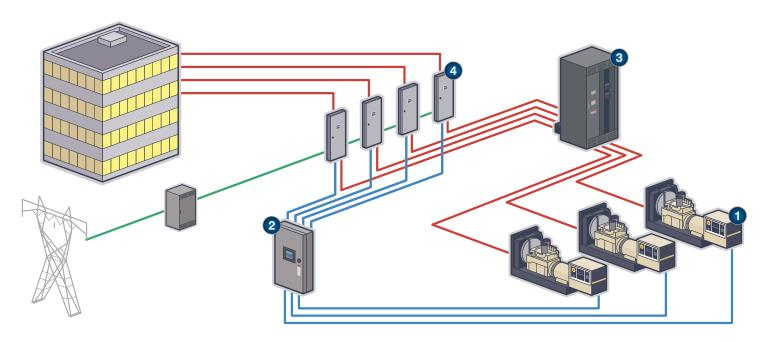
The KOHLER® Decision-Maker® Paralleling System (DPS) offers a truly integrated approach to generator paralleling. Each system includes generators, Decision-Maker 6000 controllers, a master control panel, power distribution switchboards with breakers and KOHLER automatic transfer switches.
